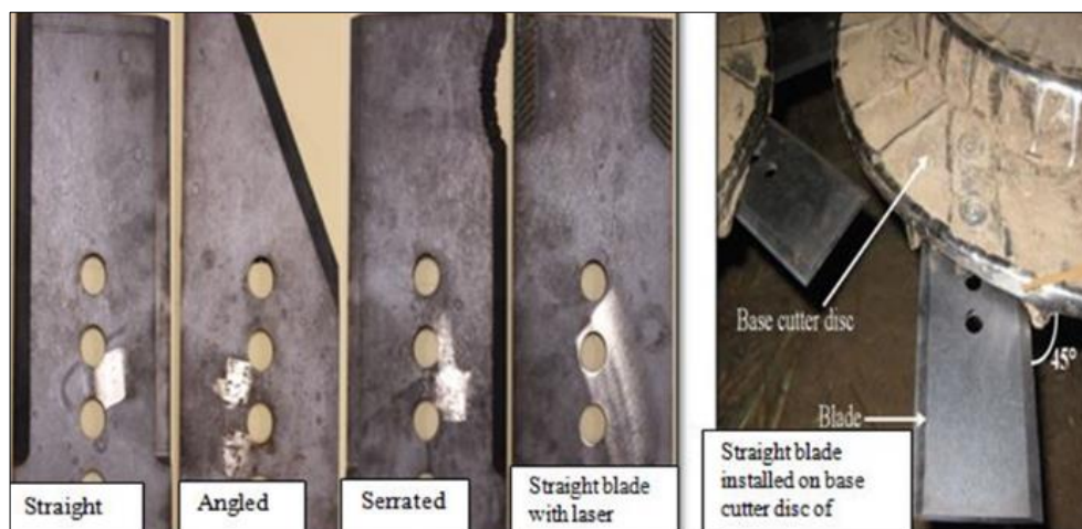
Fig 4: Four blade designs used in the experiments (Momin et al. , 2017) [32]
