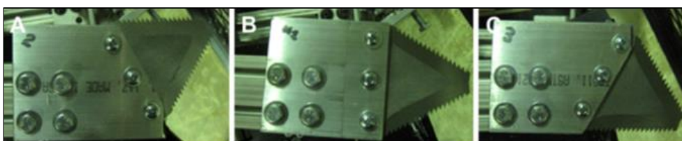
Fig 1: Serrated cutting blade mounted at different oblique angles representing: straight cut (0°) (A), 30° oblique cut (B), and 60° oblique cut (C). (Johnson et al. , 2012) [20]
