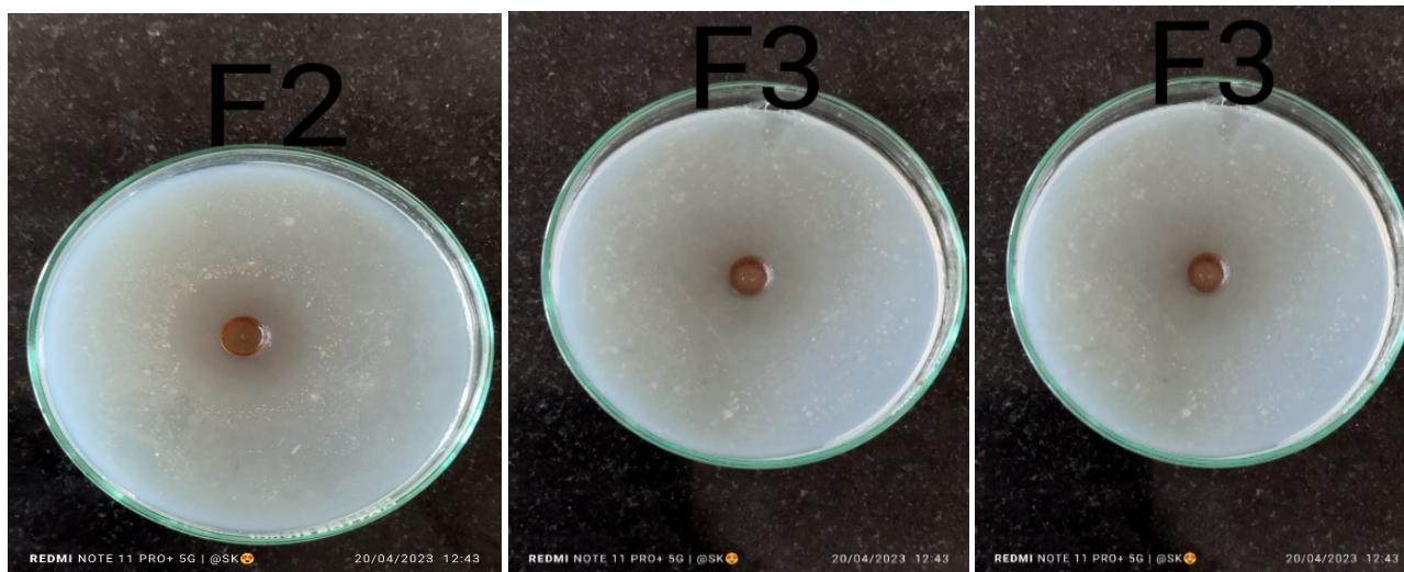
Fig 2: Evaluation of the antifungal activity against M Furfur by Well diffusion assay method
