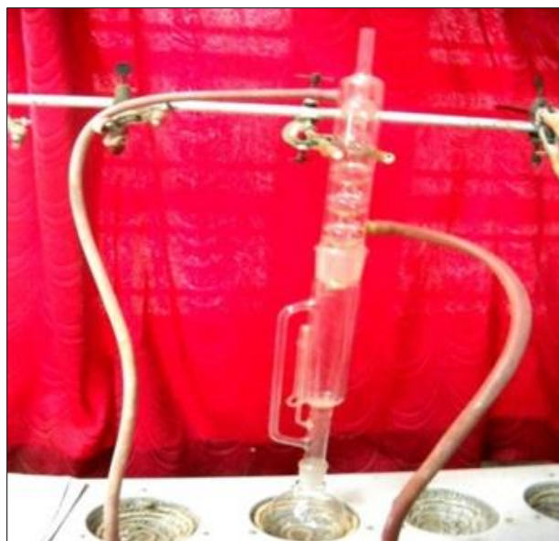
Fig 2: Soxhlet apparatus for extraction of phytochemicals
